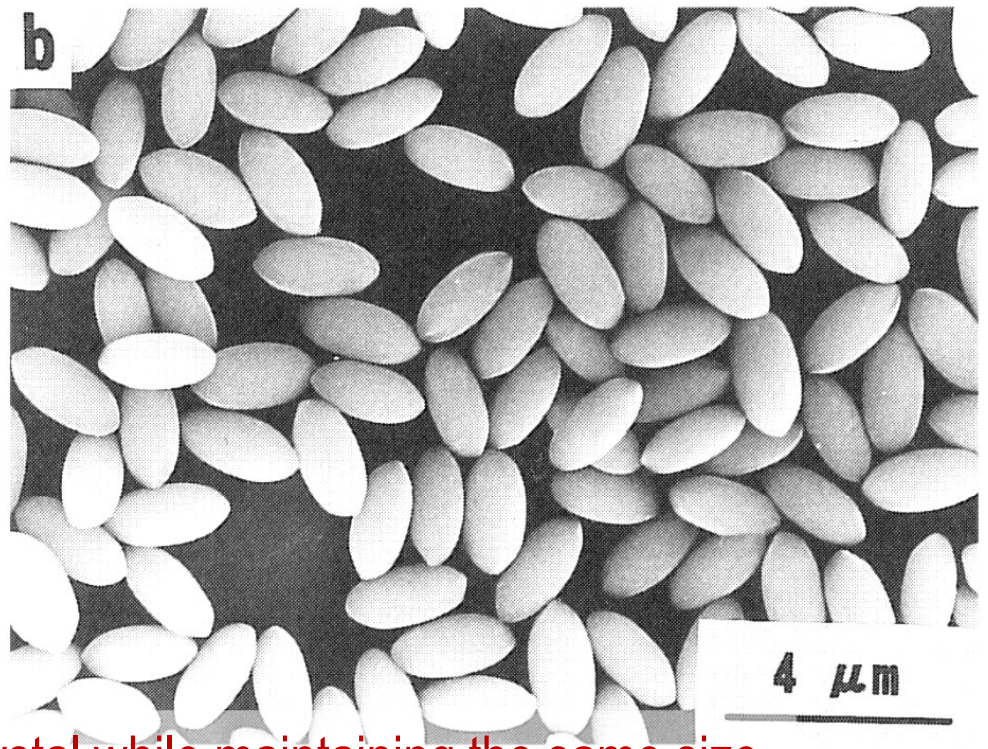
Change from polycrystalline to single crystal while maintaining the same size
