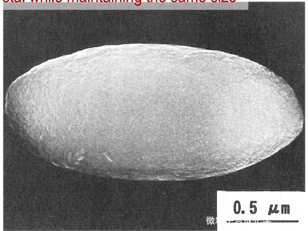
Change from polycrystalline to single crystal while maintaining the same size
